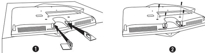
1. When installing the TV on the wall without using the stand, insert decoration covers into the holes as described in the picture ①.
